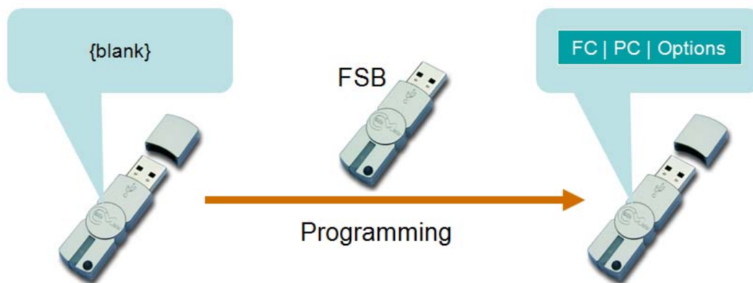
Figure 3: Programming a CmStick
