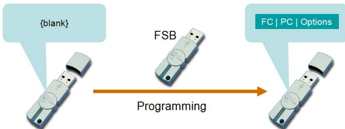
Figure 8: Programming a locally connected CmStick
